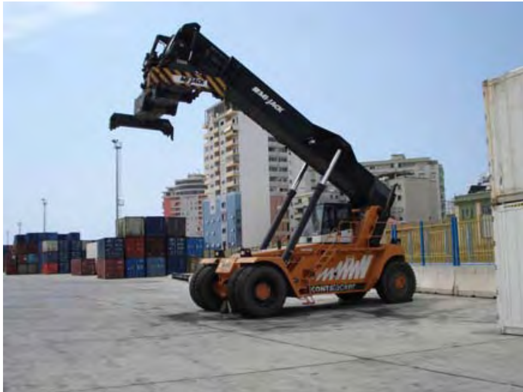
Figure 2-9 Reachstacker ne sheshin e konteniereve
